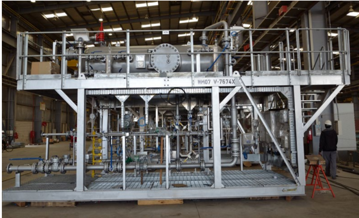
45 off Test Separator Skids (Size: 1067mm ID x 3,600 mm T/T Length; Material - SA 516 Gr.70)
