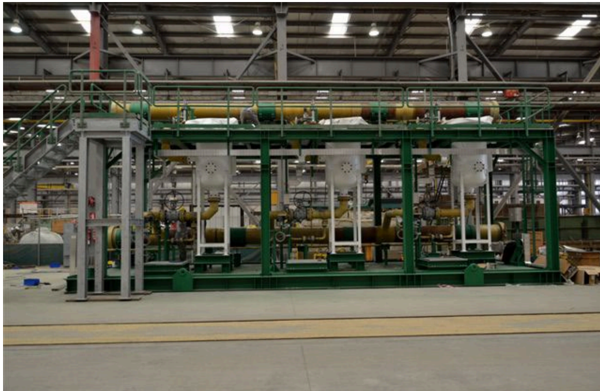
2 Cartridge Filter Skid Packages (Size: ID x 1,600 mm T/T Length; Material - SA 516 Gr.70)
