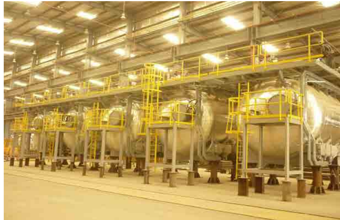
Hydromation Filter – Qty: 8 no. (Size: ID x 2996 mm T/F Length; Material - SA 516 Gr.70)
